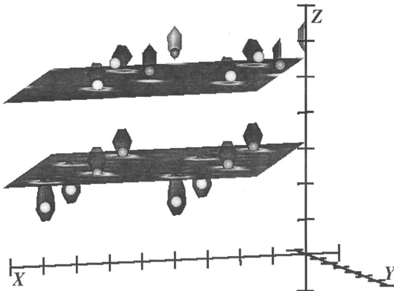
Fig. 8. High electron density isosurfaces after modification of the density distribution of Fig. 7 by the inclusion of just the (integer-order) CTRs in the iterative algorithm. Note that the isosurface lobes in the upper double layer indicate the relaxation of this layer to produce almost co-planar As and Ga atoms. Note, however, that the isosurfaces indicate a (1 $\times$ 1) periodicity parallel to the surface.
