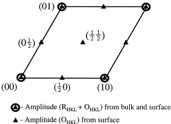
Fig. 6. Cut through reciprocal space parallel to the surface intersecting the crystal truncation rods (CTRs) specified by integer values of (HK) Miller indices, and superstructure rods corresponding to fractional values of either  $H$  or  $K$ .
