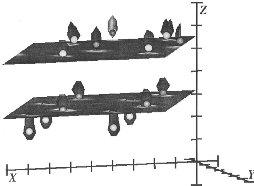
Fig. 9. Final high density isosurfaces recovered after the inclusion of both the CTRs and the (fractional-order) superstructure rods in the iterative algorithm. The true  $(2 \times 2)$  periodicity of the outermost double layer is now recovered with no high electron density in the vicinity of the vacancy at the  $z$ -axis in the outermost double layer. Note that the isosurfaces now surround just the model atom positions in this complicated reconstructed surface.
