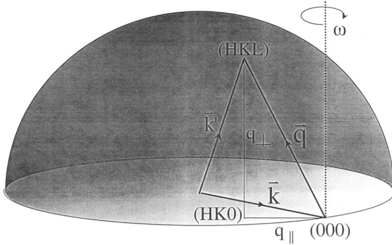
Fig. 1. Reciprocal space geometry of a surface X-ray diffraction experiment. The wavevector of the incident X-rays is represented by  $\mathbf{k}$ ; that of the diffracted beam by  $\mathbf{k}'$ . The wavevector difference,  $\mathbf{q} (= \mathbf{k}' - \mathbf{k})$  joins the origin (000) to the intersection of the Ewald sphere with the (HKL) reciprocal lattice rod ( $H$  and  $K$  are discrete, but  $L$  is continuous).
