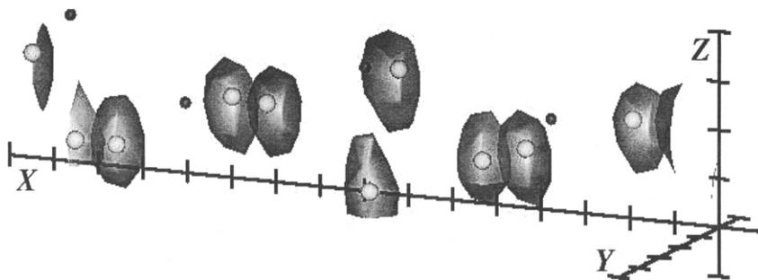
Fig. 4. Perspective view of isosurfaces of electron density representing the starting electron distribution  $\{u_0\}$  of the O/Cu(104) surface unit cell. Note that the high-density regions enclose only the substrate Cu atoms (indicated by the larger light-colored dots). No significant electron density is found in the vicinity of the O adsorbate atoms (represented by the smaller, darker dots).
