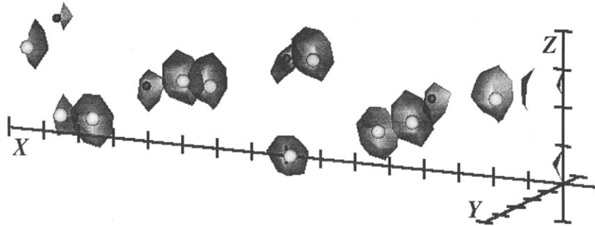
Fig. 5. Electron density isosurfaces in the same unit cell at the conclusion of the iterative algorithm. Note that now high electron density lobes are better centered around the Cu substrate atoms, and that they now also surround the O adsorbate atoms, thus revealing their positions.
